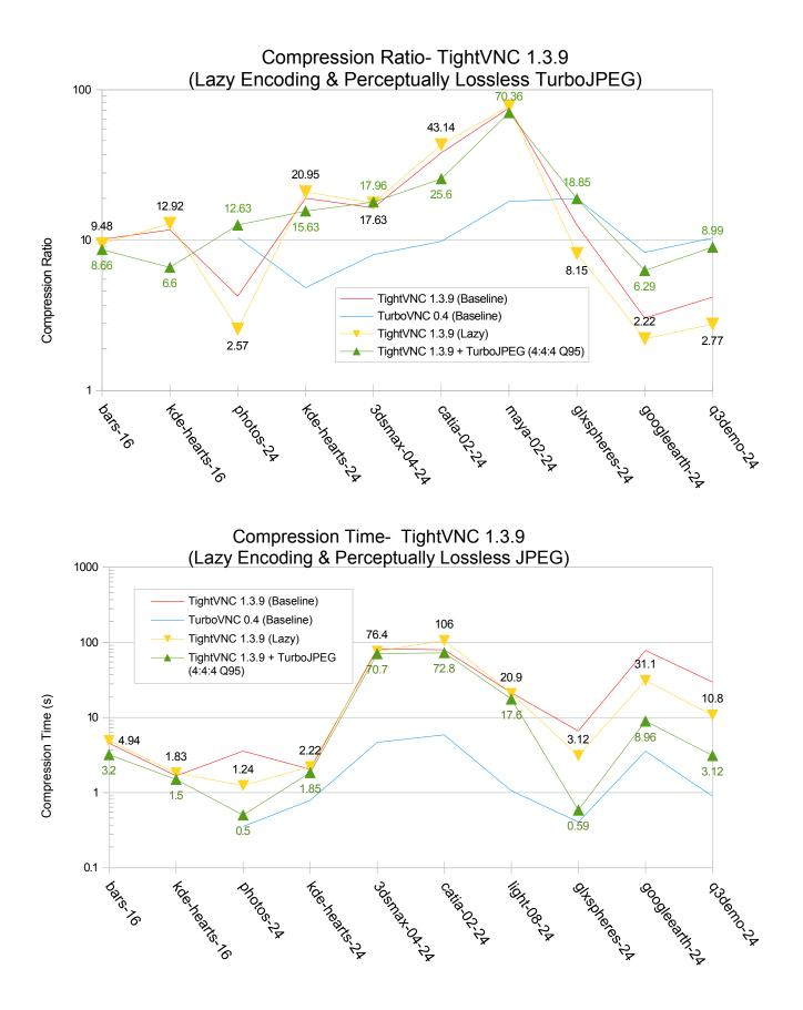
The results were mixed. The Quake 3 Demo, Google Earth, GLXspheres, and Photos datasets compressed somewhat worse but also much faster without gradient encoding. Most of the other datasets actually compressed a bit better without gradient encoding. In only one case (CATIA) did turning off gradient encoding cause a significant performance hit.
