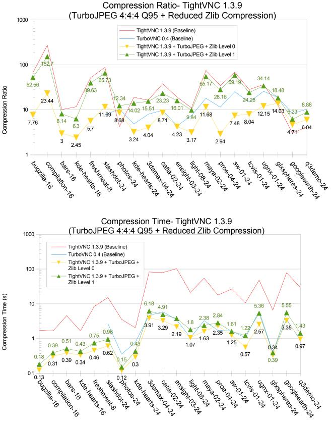
With no Zlib compression, most of the datasets exceeded the TurboVNC 0.4 performance target. However, the Quake 3 Demo and Pro/ENGINEER datasets were still slower (by 8% and 27%, respectively.) Also, most of the datasets compressed much worse than with TurboVNC 0.4.
