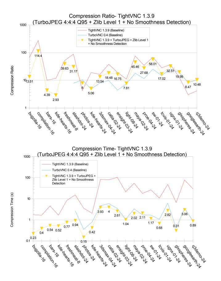
This was more like it. Almost all of the datasets compressed significantly faster and significantly better than with TurboVNC 0.4. However, the Photos dataset compressed 23% worse than with TurboVNC 0.4, and the Pro/ENGINEER dataset was slower by about 19%. Since the Photos dataset represents an important 2D workload, a regression on that dataset was unacceptable.
