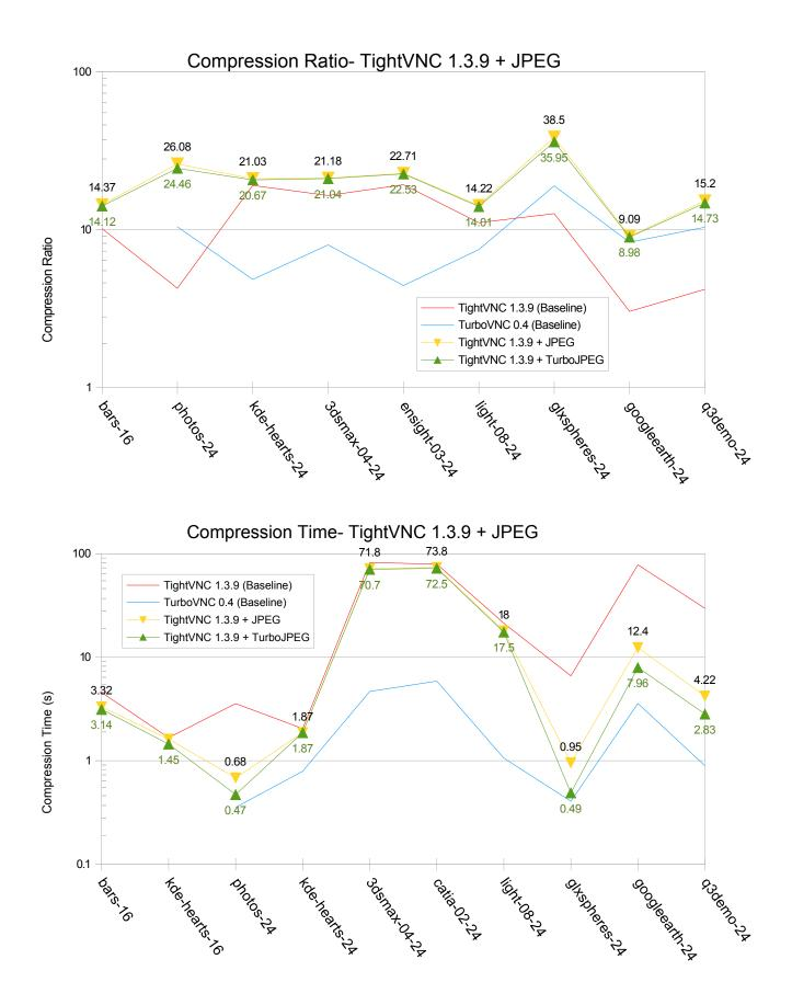
JPEG performed as fast as or faster than gradient encoding and compressed better than gradient encoding in all cases. However, the only tests that realized a significant speedup from JPEG encoding were the same four tests (Quake 3 Demo, Google Earth, GLXspheres, and Photos) that showed themselves to be good candidates for JPEG compression in the last section.
